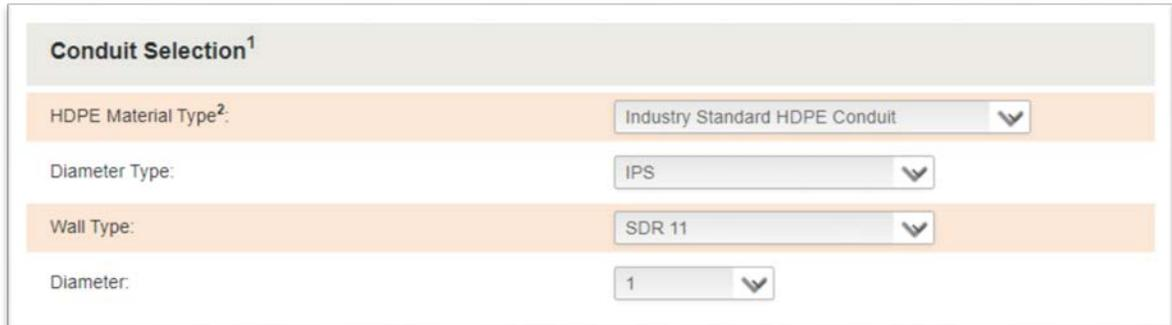
The image shows a software interface titled "Conduit Selection<sup>1</sup>". It contains four rows of input fields, each with a label on the left and a dropdown menu on the right. The first row is "HDPE Material Type<sup>2</sup>" with the selected value "Industry Standard HDPE Conduit". The second row is "Diameter Type:" with the selected value "IPS". The third row is "Wall Type:" with the selected value "SDR 11". The fourth row is "Diameter:" with the selected value "1".
